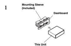
Remove the Detachable Front Panel (refer to page 6). Slide mounting sleeve from main unit (see "Removal" on page 23).
